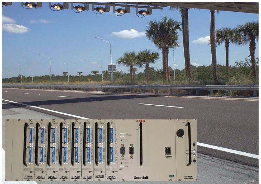
SmartToll Unit and a typical AVC tolling plaza
